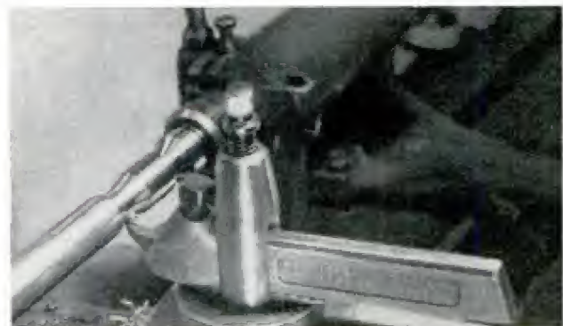
CONCAVE CUTS can be made without attachment, using bit mounted in holder and compound swing
